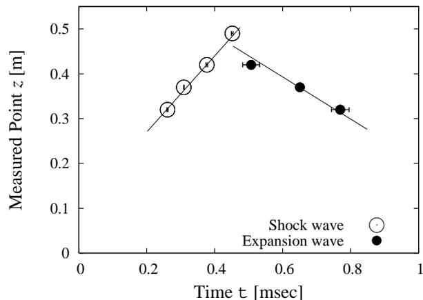
Figure 7. Relation of position of pressure gauge and arrival time.  $P=850\text{kW}$  condition.
