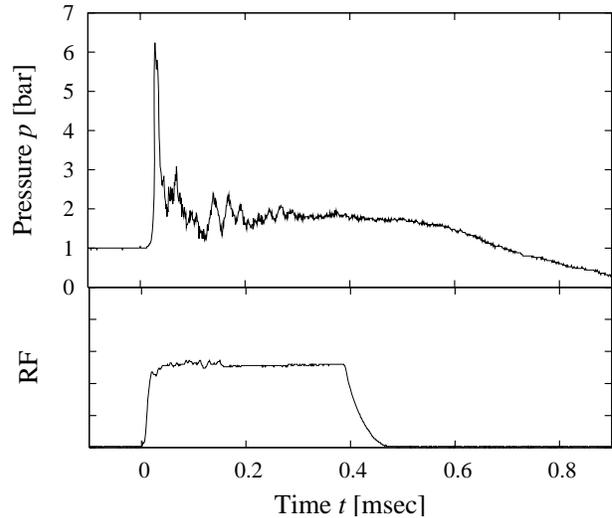
Figure 5. Typical record of pressure gauge at thruster wall.  $P=850\text{kW}$
