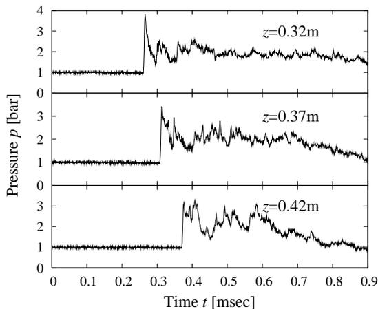
Figure 6. Typical record of pressure gauge at cylindrical part.  $P=850\text{kW}$  condition.
