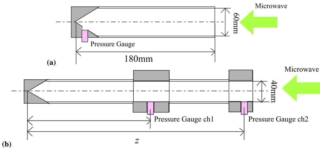
Figure 4. Schematics of pressure measurement setup.
