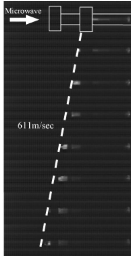
Figure 8. Photographs of plasma propagation by a high speed framing camera.  $P=630\text{kW}$  condition. 18000FPS
