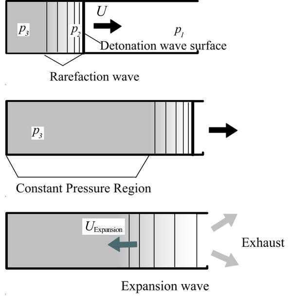
**Figure 2. Schematics of detonation engine cycle.**
