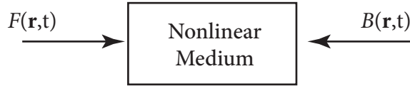
Figure 3.8: Two waves with amplitudes F(\mathbf{r}, t) and B(\mathbf{r}, t) counterpropagate within a nonlinear medium.
