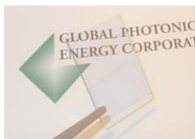
Figure 3: 100 nm of transparent Organic PV material
