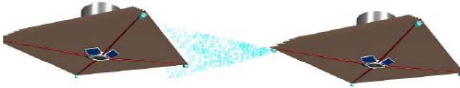
Figure 5-9. Schematic of Thruster Plume Interference with Cooled Surfaces of a Neighboring Collector Spacecraft
