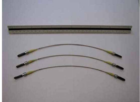
Figure 4-3. Second Set of Three Long-Fiber Single-Mode Chalcogenide Fibers Delivered by the Naval Research Lab
