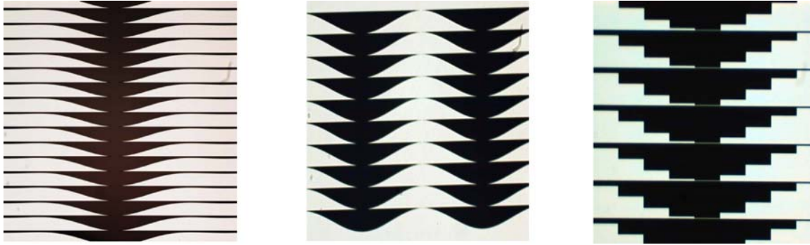
Figure 3-3. Binary 1-sinc 2 mask (left) produced by e-beam lithography of aluminium on glass for f/28.55 and a wavelength 785 nm, binary continuous sin 2 mask pattern (middle), and binary discontinuous sin 2 mask pattern (right).
