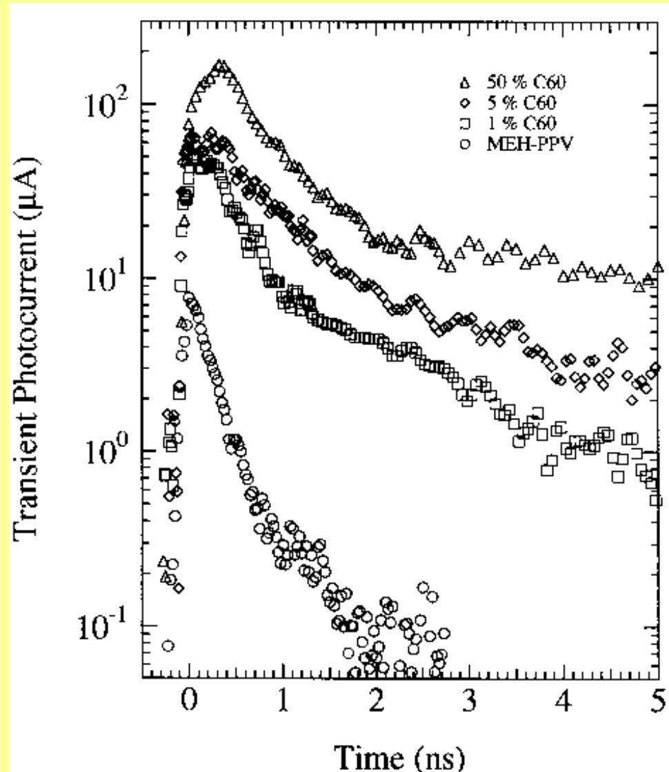
**Peak Photocurrent as well as the lifetime of the charge carriers are enhanced upon increasing the C<sub>60</sub> content in the composite.**
