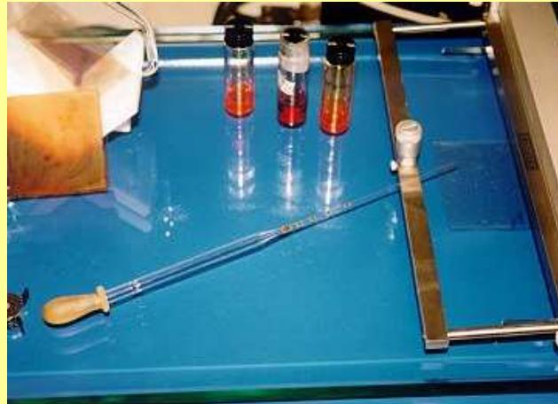
Doctor Blade Technique was developed for large area coating
